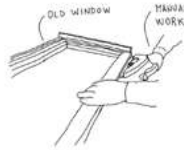
Execution of the milling to insert the colored gasket of a window.
