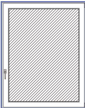
Typology: C Measure: 135 cm X 170 cm Surface: 2,3 m 2 Weight: 46 kg Material: Wood
